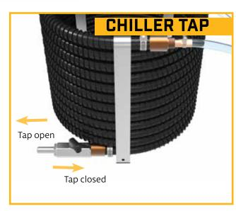
When the wort is being chilled. Adjust the tap to change how fast the wort flows through the chiller. The slower the wort runs through, the cooler it will come out
