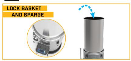
Allow the mash liquid to drain into the boiler, gently press the top perforated plate down (12) until it comes to rest against the grain. Gently pour the prepared sparge water over the grain. Keep the water level approx 10 mm (0.4 in) above the plate at all times for an even sparge. **NOTE**: Discard the used grain responsibly, it can make great compost or chicken feed.
