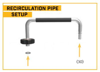
Take one of the recirculation pipe O rings (33) from the small clear bag and place it over the bottom of the recirculation pipe (1) and push the plastic knob down over the O ring. Then put the silicone reticulation hose (30) over the barbed end of the recirculation pipe.
