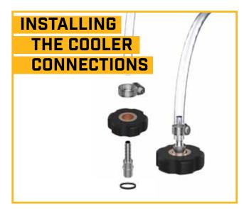
From the bag with the chiller connections, place one of the O rings (26) over the bottom end of the barbed nipple. Take hose clamp from connection D (but leave hose attached). Take the free end of hose A (shortest hose) and push hose clamp (taken from connection D) onto the end. Push the barbed nipple (25) through the hole in the plastic knob (24). Push hose A with the hose clamp onto the barbed nipple with plastic knob and secure.
