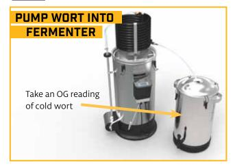
Turn the cooling water on. Once the 'cold wort out' hose runs cold switch the pump 'Off' and place it inside the clean and sterilised fermenter. Adjust the chiller tap to control the temperature of the wort flowing into the fermenter. Always try to keep the fermenter sealed. Add yeast as instructed on recipe.
