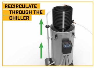
Connect the counter flow wort chiller as you would normally. Set the controller temperature to 55°C (131°F). Place the 'cold wort out' (connection D) hose from the chiller through the hole in the glass lid and let the cleaner recirculate through the chiller for 5 minutes.
