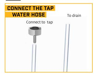
The two long hoses on the chiller (connection B and C) are the cooling water hoses. Connect hose B to your tap adaptor. Hose C is where the water drains out. This will come out hot as the water flows through the chiller.
