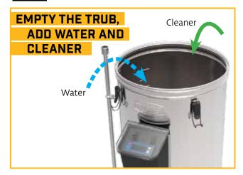
Empty out the trub by tipping it down a drain. Remove the pump filter and rinse it, replace it again after rinsing. Fill the boiler up with 7.5 L (1.98 US Gal) of water. Add 30 ml (1 oz) of cleaner.
