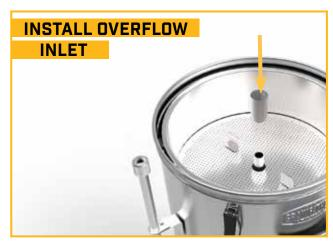
Fit the overflow inlet (20) onto the overflow top pipe (21) and press down until it fits into the hole in the top perforated plate (12).
