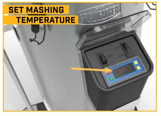
Input the temperature you want to mash at making sure the 'Mash'/'Boil' switch is in the 'Mash' position. Ensure the element variation switch is in the "Normal" position.
