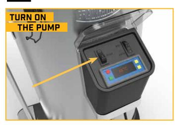
Switch on the pump. The wort flowing through the recirculation pipe should fill up on top of the top perforated plate.
