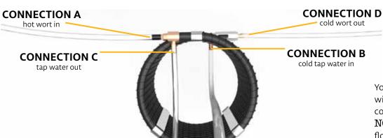
Your counter flow wort chiller will come with 4 hoses already connected to connections A B, C and D.
